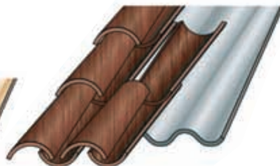
Double aligned installation with peak and trough tiles
