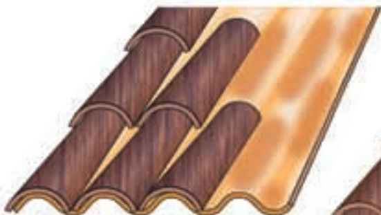
Simple aligned installation with peak tiles only
